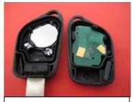
Once you open your remote you end up with bottom part and top part consisting electronics and plastic button shell.
