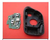
You should end up with electronic board part and hard plastic shell free of old buttons, ready for inserting new silicone buttons in.
