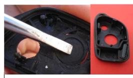
Old rubber buttons should be removed by pushing it through with the small screw driver. If any remnants of an old buttons are still left around holes they need to be scraped off/cut out with Stanley knife. Be careful not to damage plastic shell.
